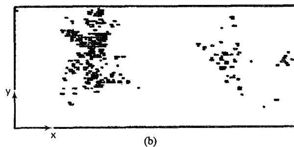
Fig. 7. Microwave cross-polarized transmission C scan of carbon inclusions and voids in reaction-sintered \text{Si}_3\text{N}_4 . Frequency=92.6 GHz. (a) Amplitude versus position. (b) Excess signal versus position.
